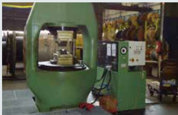
Hydraulic wire rope swaging press 3,000 tons
